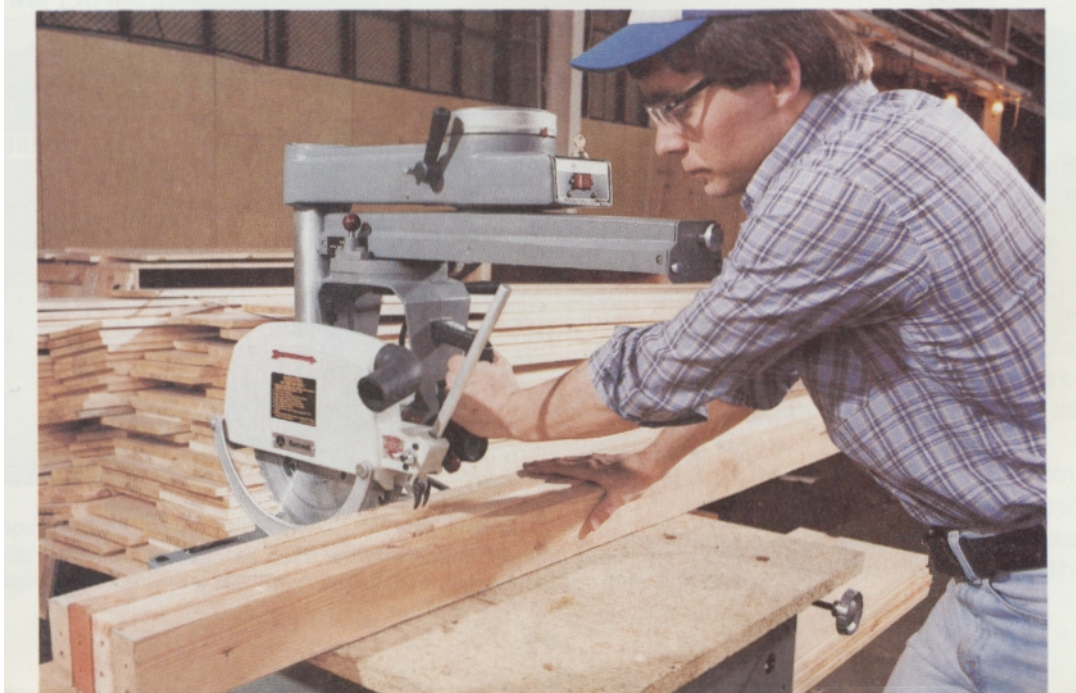
Fig. 3-30. Using a radial arm saw to cut dimension lumber. Material of this size would be difficult to slide through a table saw. (Delta International Machinery Corp.)
