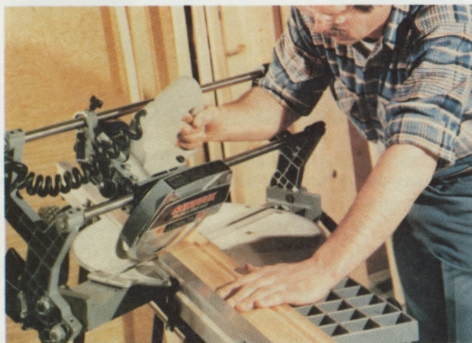
Fig. 3-41. Sawbuck frame and trim saw being used to make a compound miter cut. It crosscuts, miters, bevels, and makes compound cuts on any stock up to 2 x 12. (Delta International Machinery Corp.)
