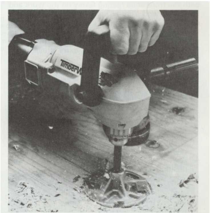
Fig. 3-15. Pressure required to operate a drill will vary with drill size, type of wood, and diameter of the drill bit. This drill is operating a bit cutting a large diameter hole. (Black & Decker Mfg. Co.)
