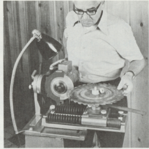
Fig. 3-42. Skilled worker sharpens carbide tipped circular saw blade. (Foley Mfg. Co.)
