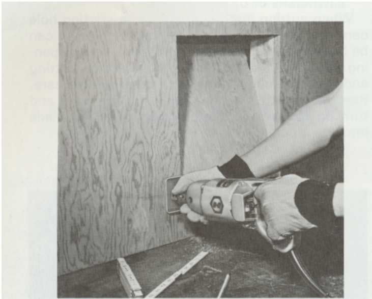
Fig. 3-11. Heavy-duty reciprocating saw operation is much like the saber saw. (Black & Decker Mfg. Co.)
