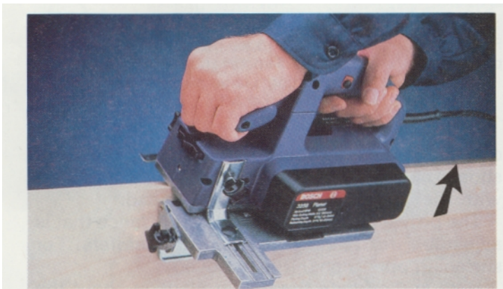
Fig. 3-17. Portable power plane is being used to plane a chamfer. Note arrow. (Bosch Power Tool Corp.)
