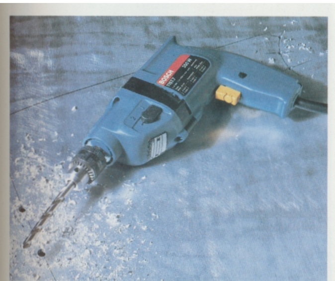
Fig. 3-14. Variable speed electric drill. Direction of rotation can also be reversed. No-load speed can be varied from 0 to 1500 rpm. (Bosch Power Tool Corp.)
