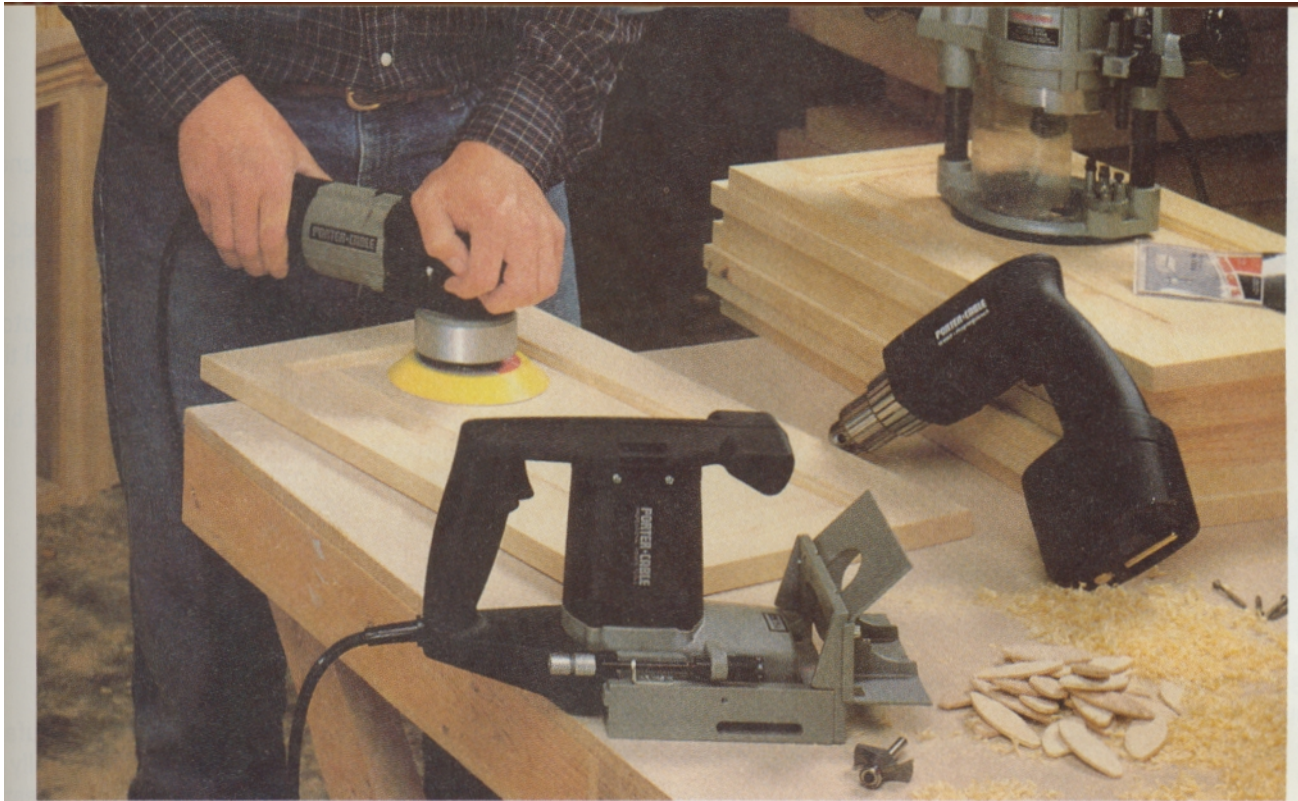
Portable power tools are used in every stage of construction. New and improved units are continually being developed. In the view above, an orbital sander is being used to smooth a cabinet door. Clockwise around the view is a plunge router, a cordless drill, and a plate joiner. The plate joiner cuts slots in the edges and ends of stock to be joined. Wooden biscuits (shown in the view) are inserted in the slots and the assembly is glued together in about the same way as dowel joints. (Porter-Cable Corp.)
