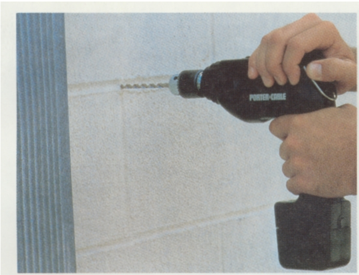
Fig. 3-16. Cordless drills are useful where power is not easily available. This one is drilling a hole in masonry. (Porter Cable)
