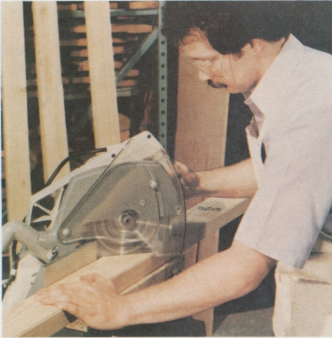
Fig. 3-40. Using a power (motorized) miter box to make an angle cut on a 2 x 4. Cuts can be made either to the right or left as with a regular miter box.
