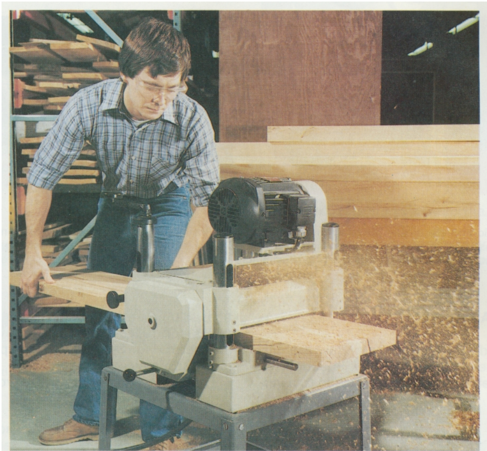
Stationary planer is small enough to take onto a construction job. This unit will plane stock up to 13 in. wide and nearly 6 in. thick. (Delta International Machinery Corp.)
