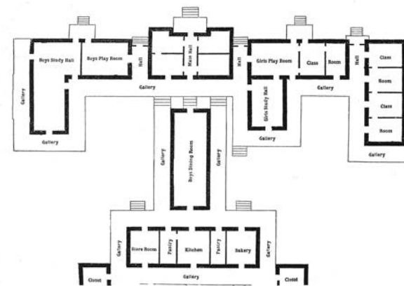
Left: The plan of the TSD Main Building upon completion of renovations and additions designed in 1883 by Taylor & Williams developed a network of buildings connected by three stories of promenade galleries that would remain in place until the building’s demolition in 1956.
